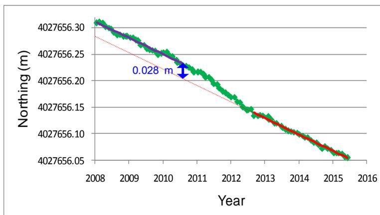
**Fig. 3** Time-series of Northing of station 048A and its displacements due to the volcano inflation.
