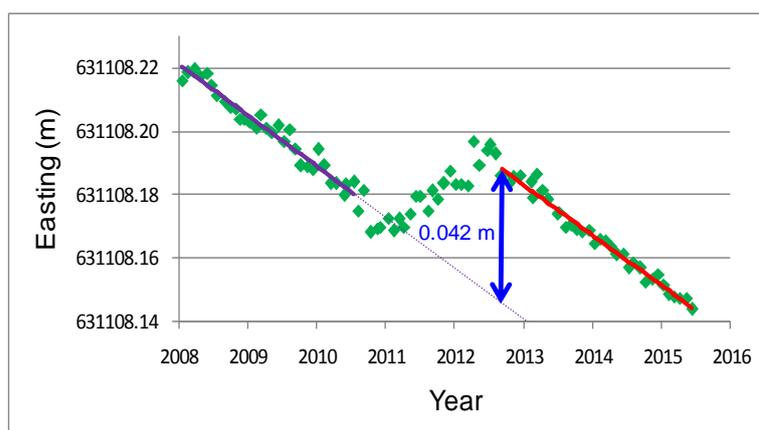
**Fig. 2** Time-series of Easting of station 048A and its displacements due to the volcano inflation.
