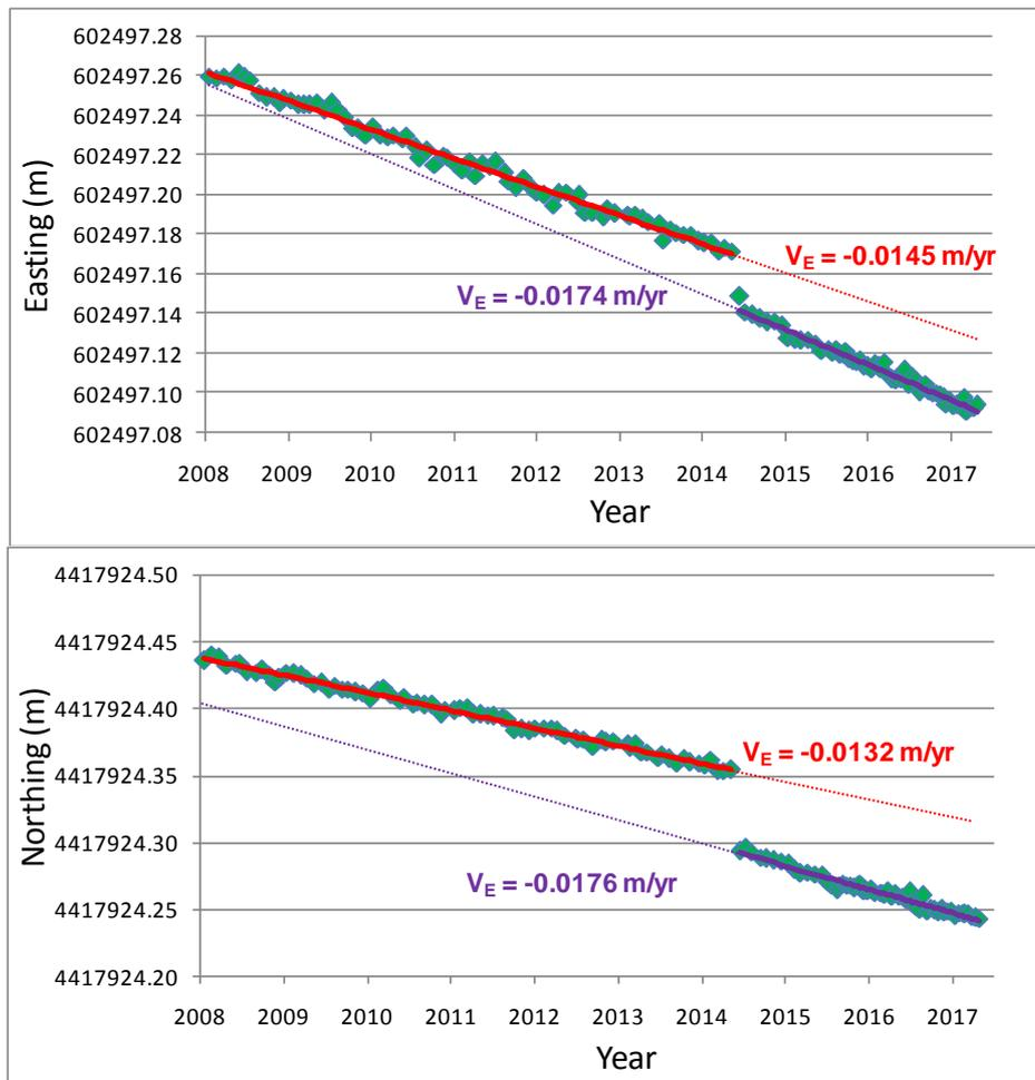
**Fig. 8** Coordinate time-series for station 089A and estimated velocities before (in red) and after the earthquake (in purple).
