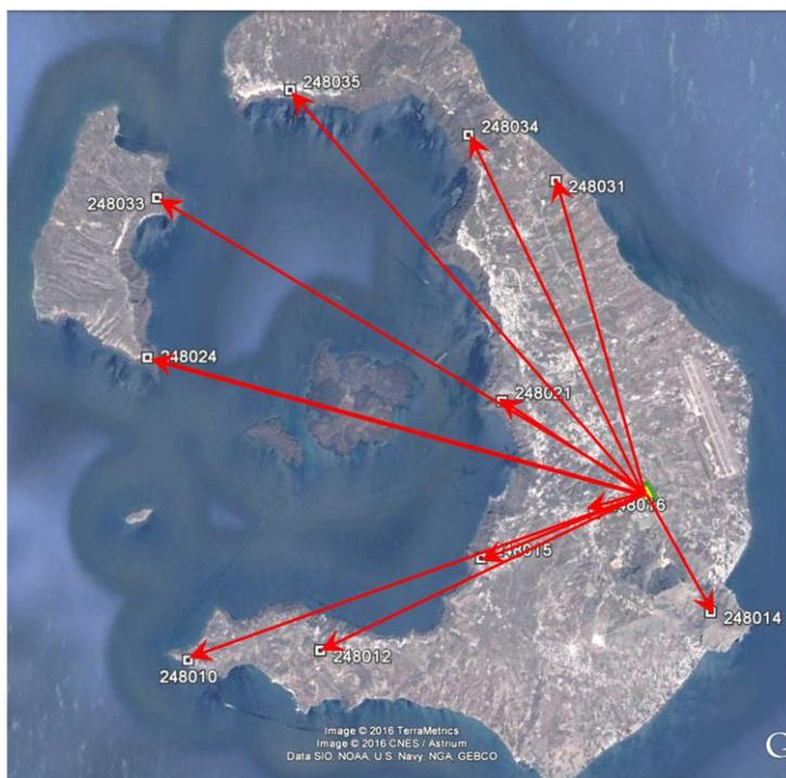
**Fig. 1** The locations of the 11 benchmarks and the measured baselines.
