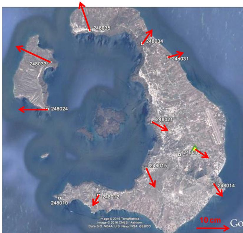
**Fig. 6** The displacement vectors (final results after excluding problematic points).
