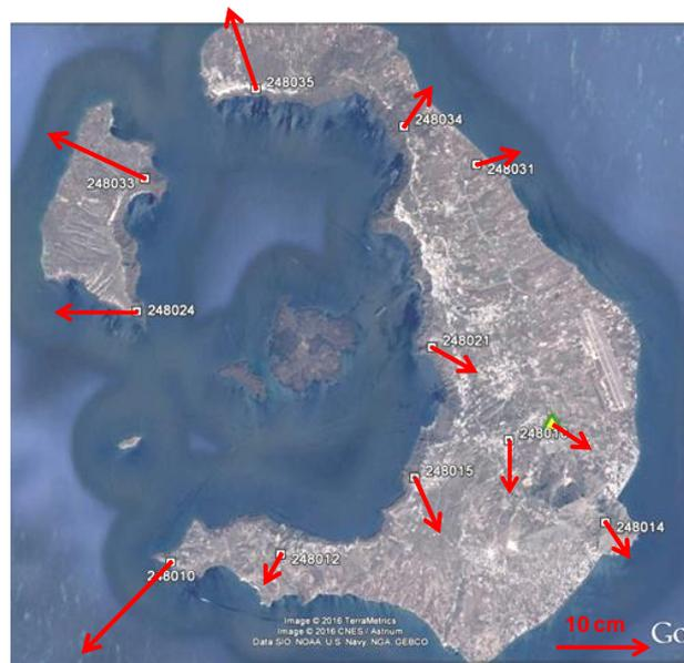
**Fig. 4** Displacement vectors (initial results).
