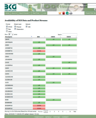
Fig. 7: The availability of the data and combination products streams is monitored for all three IGS broadcasters. Currently, short and long mount-point names are used in parallel. For the three EUREF regional broadcasters at ASI, BKG and ROB a more sophisticated monitoring showing some more details, e.g. format type, last connection etc. is implemented at the EPN Central Bureau on http://www.epncb.oma.be/_networkdata/data_access/real_time/status.php .
